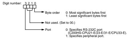
The specified number of bytes will be read from S through S+(NP2)–1 and transmitted through the specified port.
